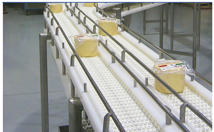
Sanitary conveyor systems are designed for agency compliance with stainless steel construction and are built to food industry and plant specific needs as dictated by sanitation or food safety requirements.
