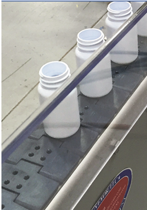
Vacuum conveyors utilize blowers or an enclosed fan to move air beneath the conveyor to cause a suction effect through a perforated conveyor belt.
